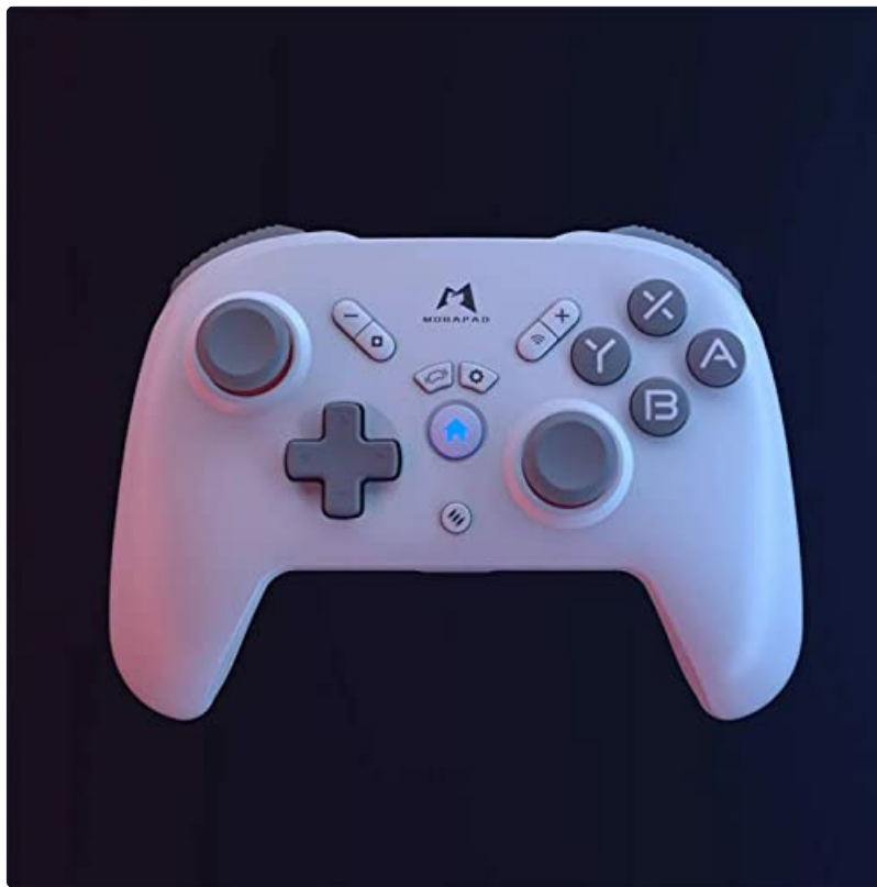
Image: Front view of the Mobapad M073 controller, showing the left and right joysticks, D-pad, A/B/X/Y buttons, Home button, Capture button, Plus/Minus buttons, and other function buttons.
