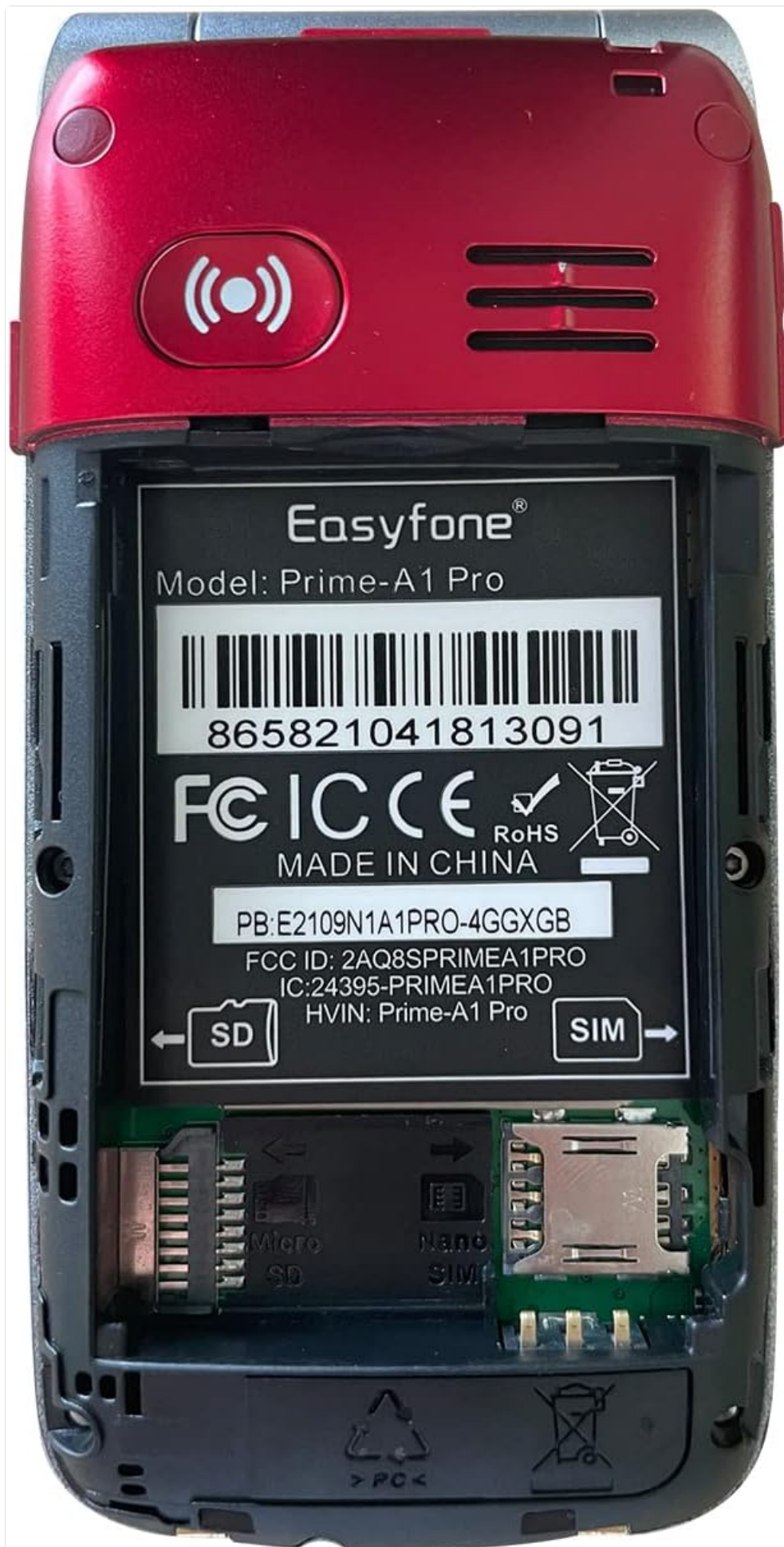
Figure 4.1: View of the phone's interior showing SIM and Micro SD card slots.
