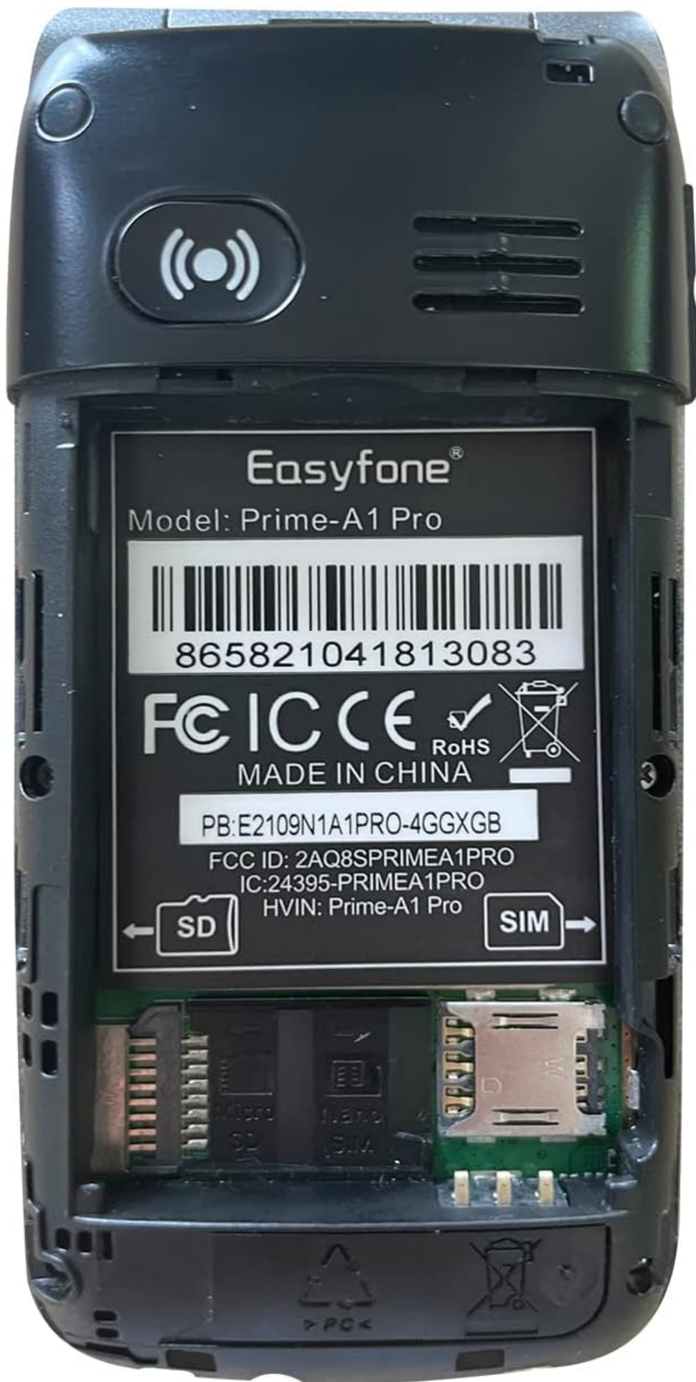
Image: The internal compartment of the phone, illustrating where to insert the SIM and SD cards.
