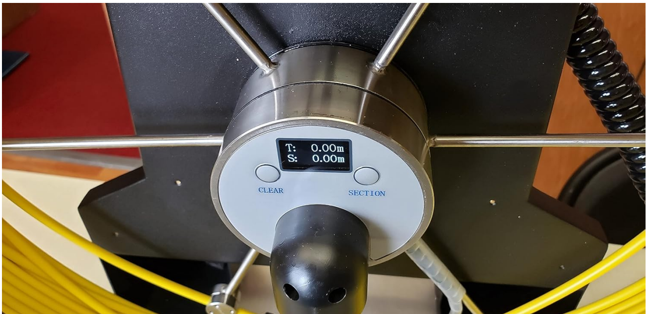
Figure 7: Control unit buttons for photo and video recording functions.
