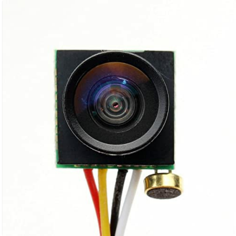
Front view of the REES52 600TVL Mini FPV AV Camera, showing the wide-angle lens and integrated microphone.
