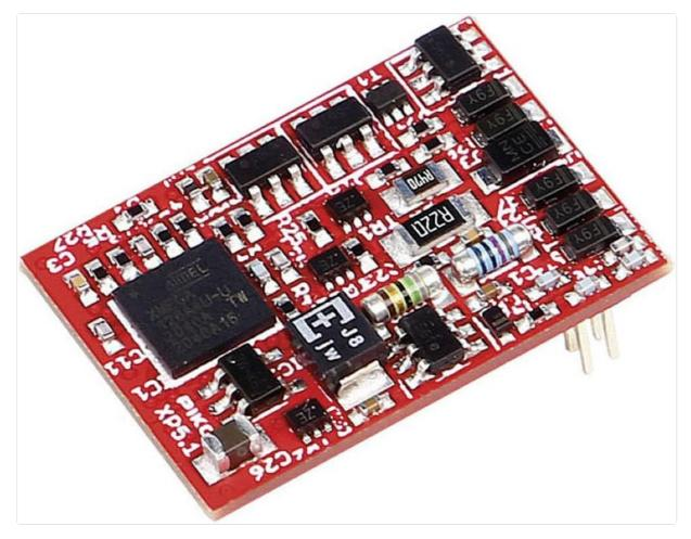
An overhead view of the Piko 56502 Smart Decoder XP 5.1, a compact red circuit board with various electronic components including integrated circuits, resistors, and capacitors. A multi-pin connector is visible on one side.
