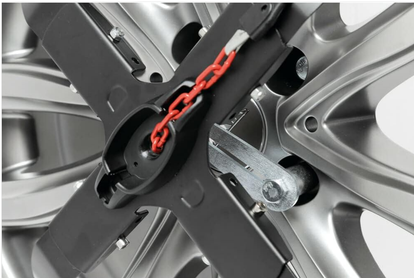
Figure 3: A closer look at the secure attachment of the snow chain to a hexagonal wheel bolt, highlighting the robust connection.
