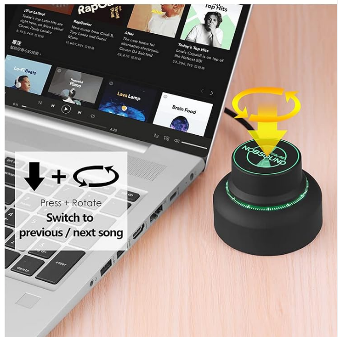
Figure 6: Operational Controls. An instructional diagram demonstrating the core functions of the Nobsound Vol-02. It shows pressing the knob for mute/unmute, rotating it to adjust volume, and pressing while rotating to skip tracks (previous/next).
