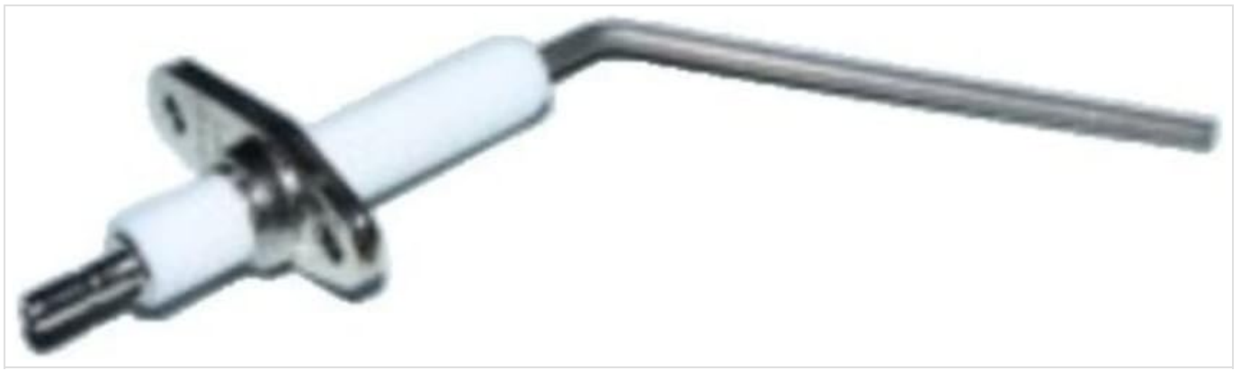
Figure 1: Sime Murelle HE25.55 Ionization Probe. This image shows the probe with its ceramic insulator and metal electrode, designed to be inserted into the boiler's combustion area. The metal bracket with screw holes is visible for mounting.
