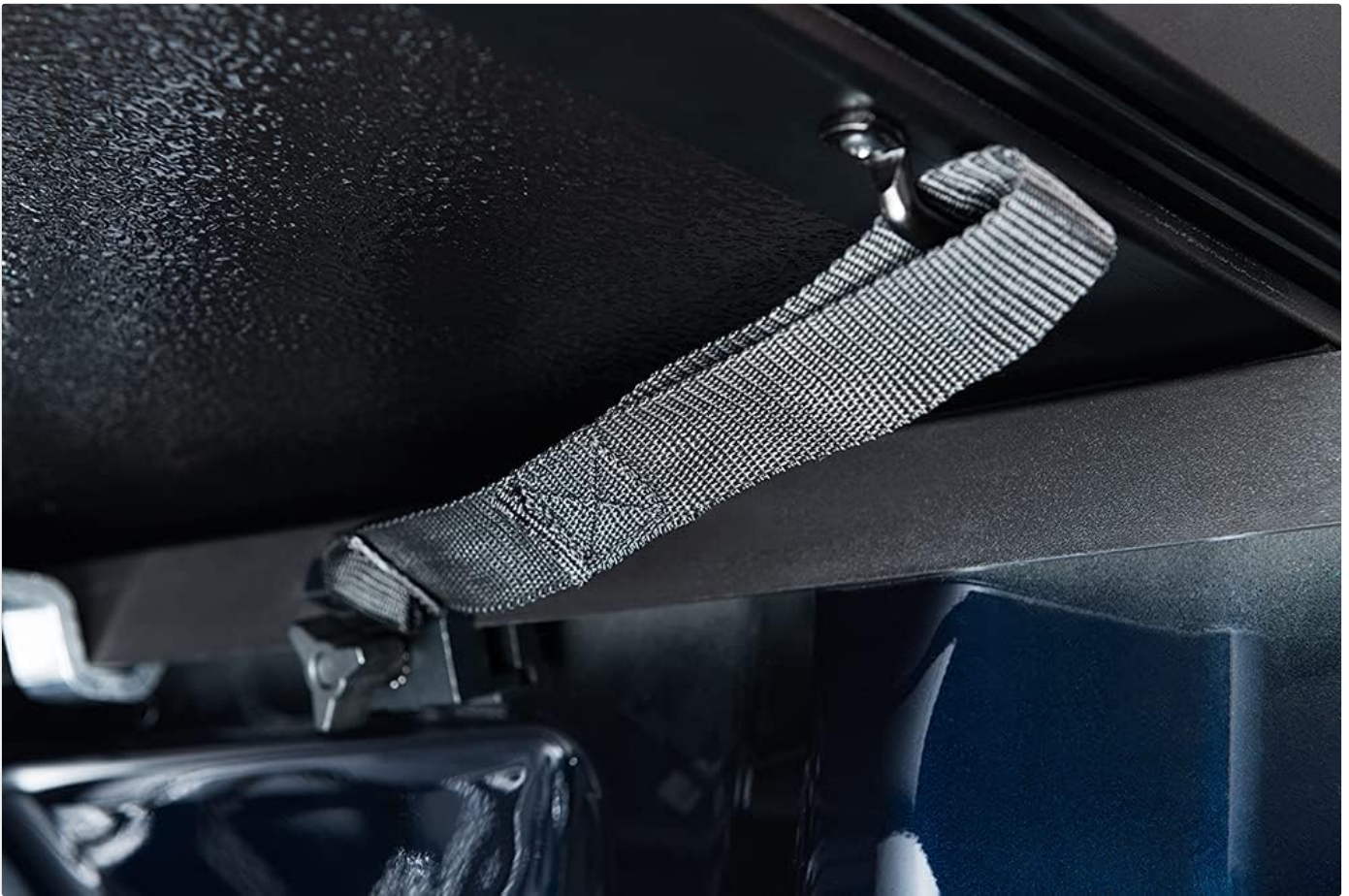
Image: A close-up view of the securing strap, used to hold the tonneau cover in its folded, open position against the truck cab.
