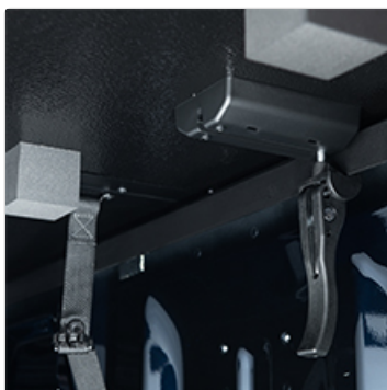
Image: Underside view of the tonneau cover, illustrating the latch and clamp mechanism used to secure the cover to the truck bed rails.
