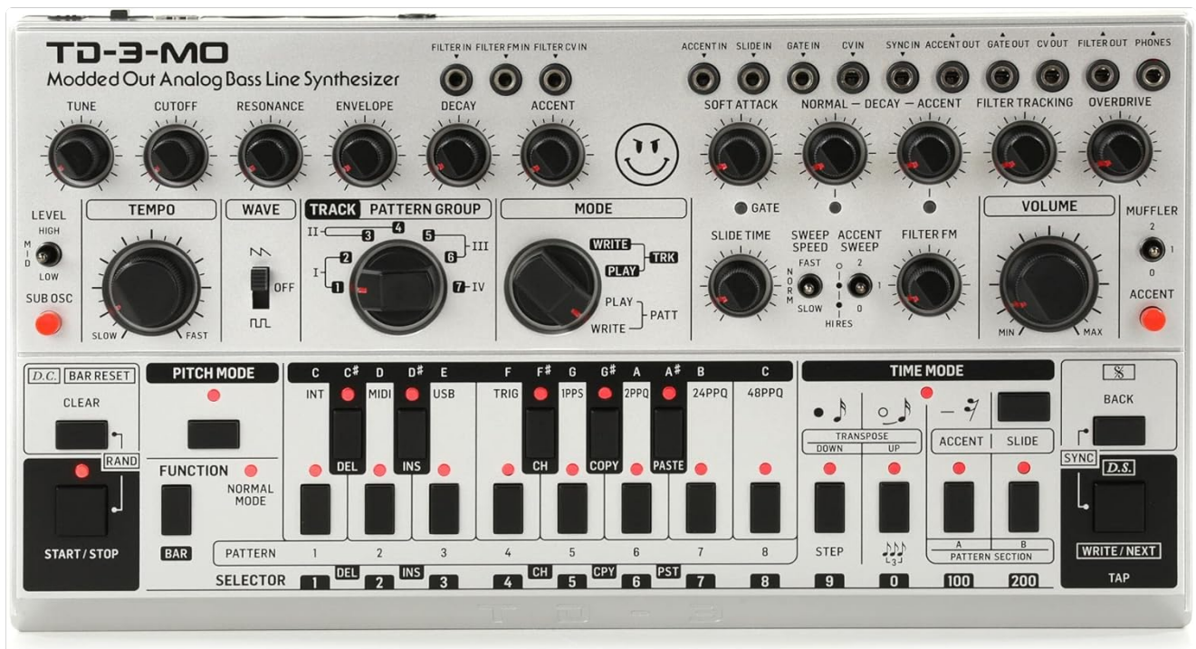
Figure 4.1: Front panel layout of the Behringer TD-3-MO-SR Analog Bass Line Synthesizer, showing all knobs, switches, and buttons.
