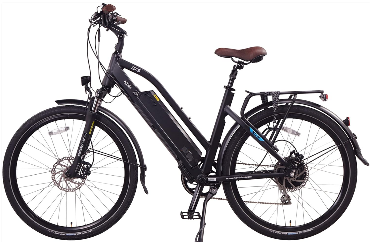
Figure 3.3: Side view of the NCM Milano Plus, showing the battery compartment, motor, and disc brakes.
