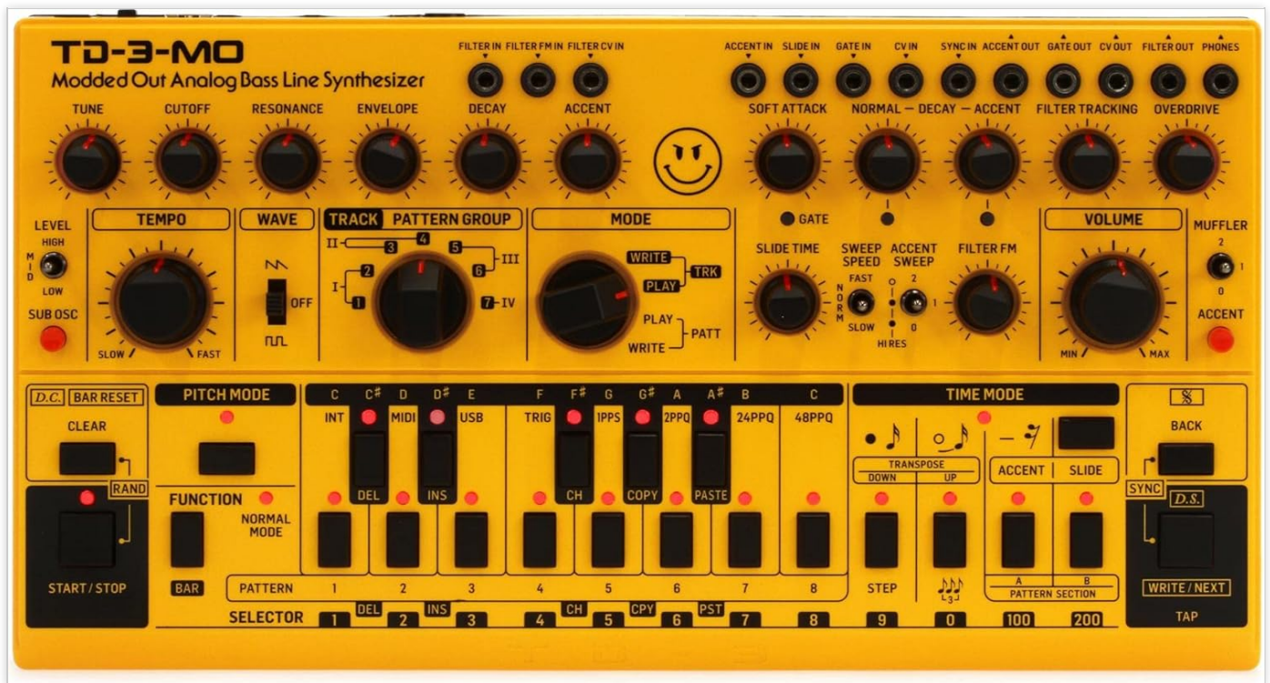
Figure 1: Front panel of the Behringer TD-3-MO-AM Analog Bass Line Synthesizer. This image displays all knobs, buttons, and input/output jacks, including controls for Tune, Cutoff, Resonance, Envelope, Decay, Accent, Tempo, Wave, Track/Pattern Group, Mode, Gate, Slide Time, Sweep Speed, Filter FM, Volume, and various input/output ports.
