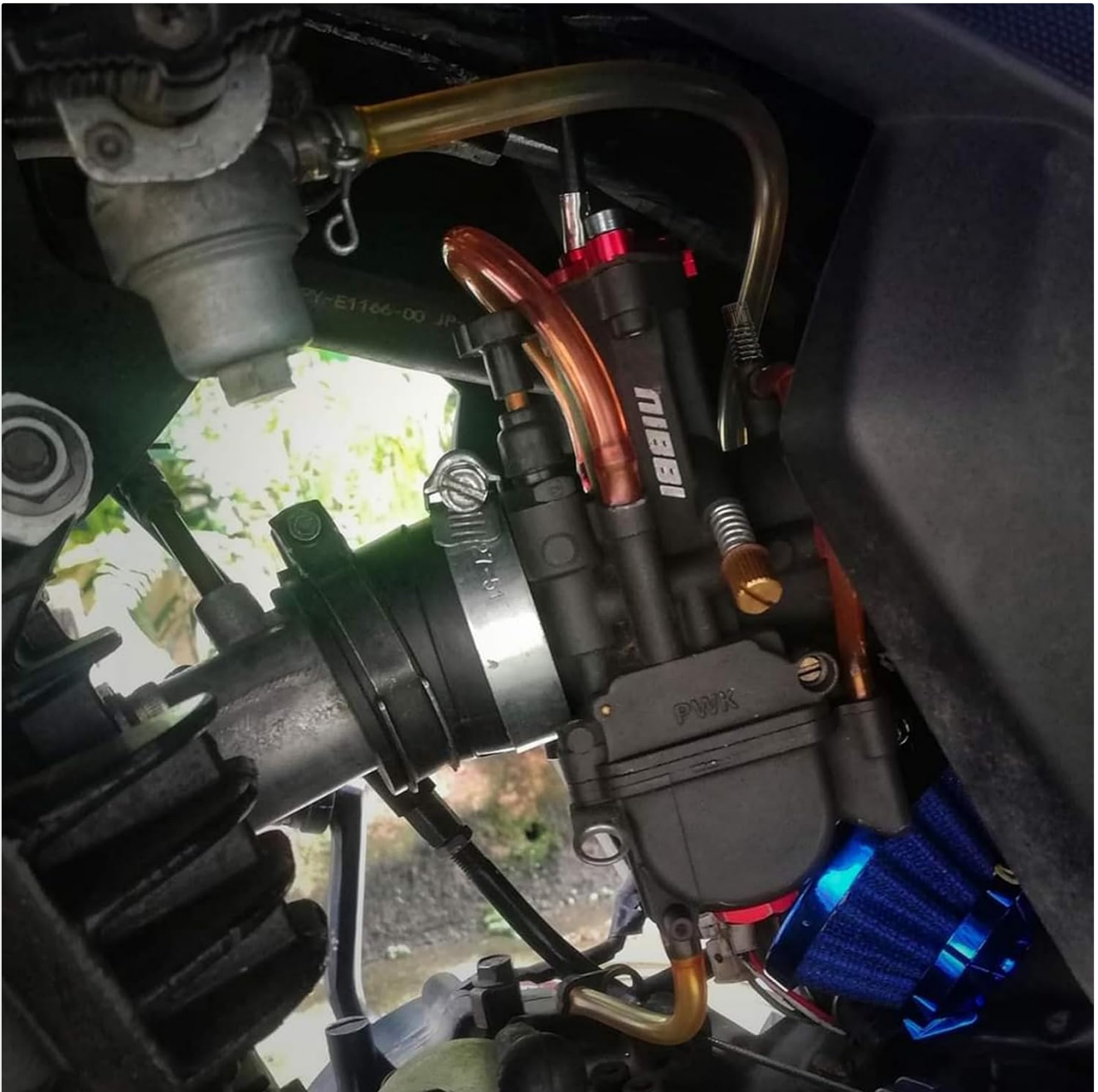
Image 2: NIBBI PWK34 Carburetor shown installed on a motorcycle engine.
