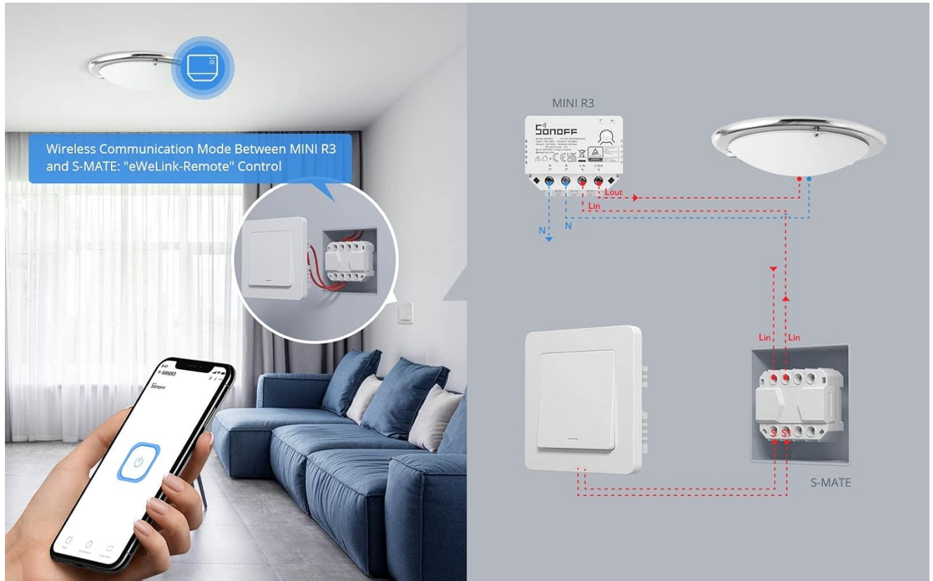
Image: Diagram illustrating the wireless communication between SONOFF MINI R3 and S-MATE for eWeLink-Remote control.
