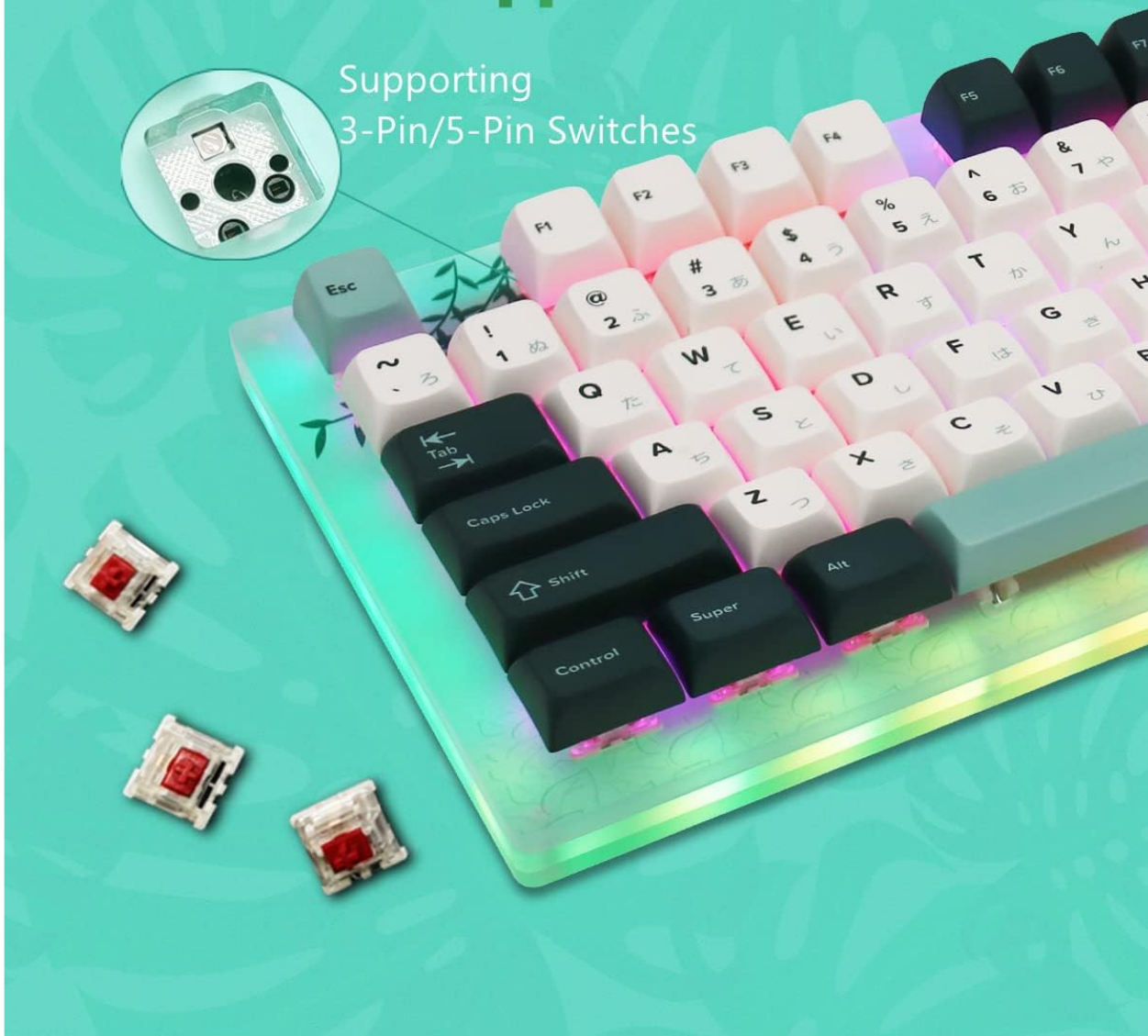
Image 4.3: Illustration of the hot-swappable switch feature, supporting 3-pin/5-pin switches.
