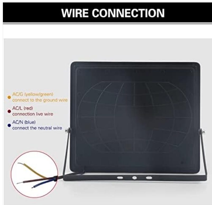
Image 4: Wire Connection Diagram. This image provides a clear guide for connecting the floodlight's wires: yellow/green for ground, red for live, and blue for neutral.
