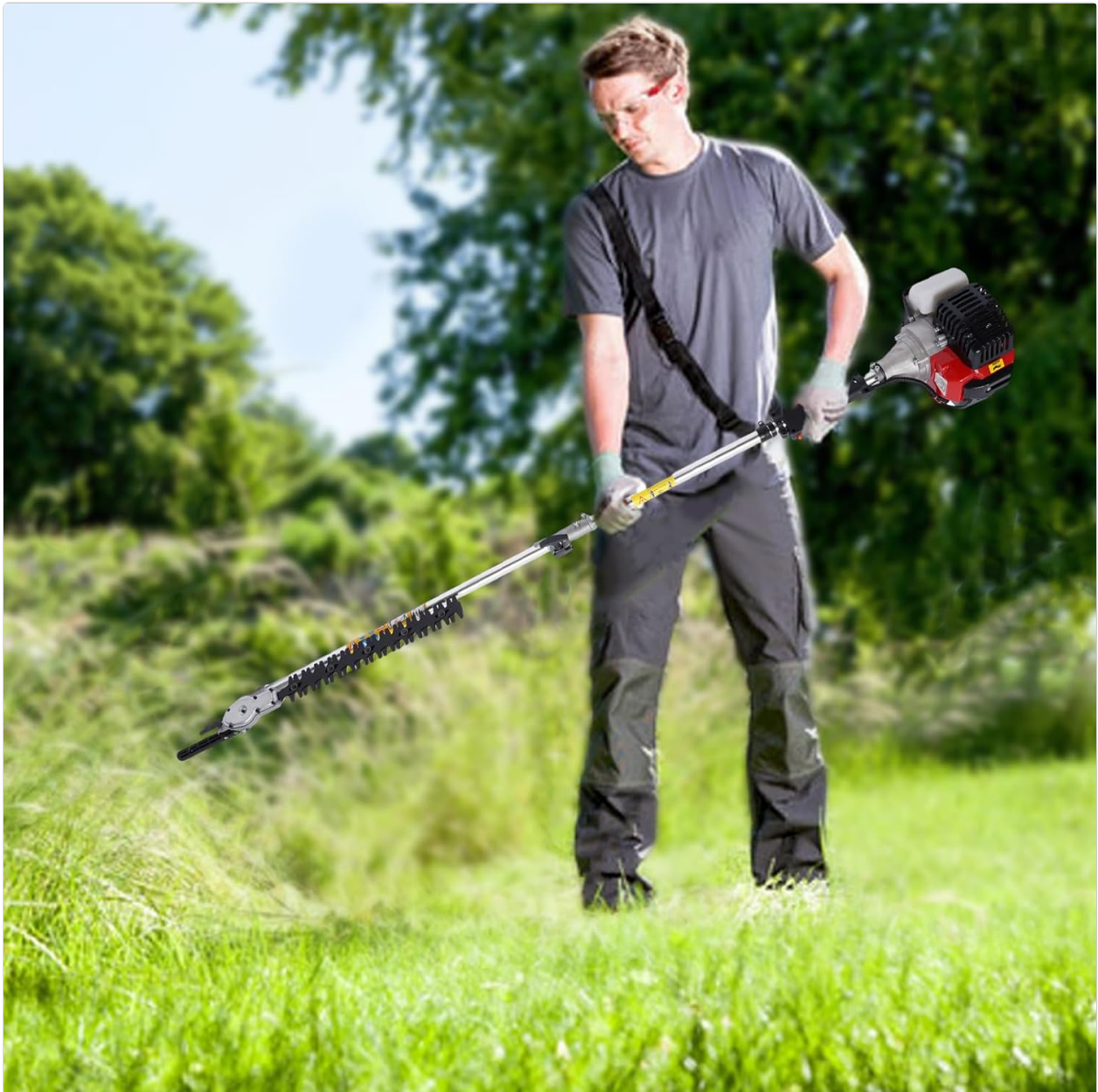
Image 2.1: Always wear appropriate safety gear, including eye and ear protection, when operating the tool.
