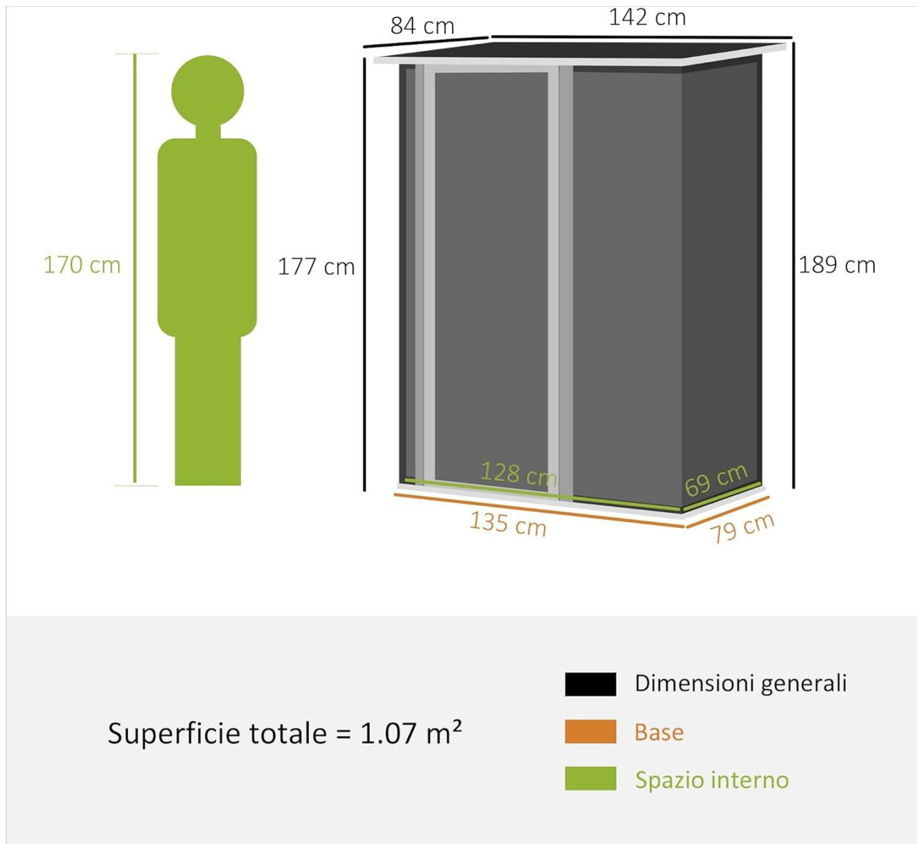
**Image Description:** A diagram illustrating the overall dimensions of the shed: 142 cm (Length), 84 cm (Width), and 189 cm (Height). It also shows internal base dimensions and total surface area.
