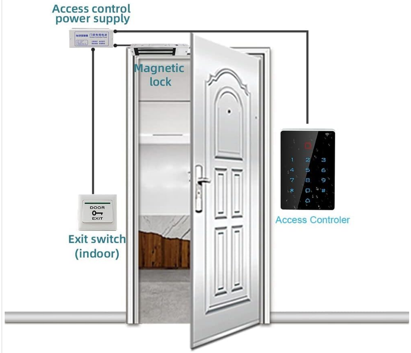
Figure 3: Typical product usage diagram illustrating the connection of the access controller with a magnetic lock, power supply, and an indoor exit switch.
