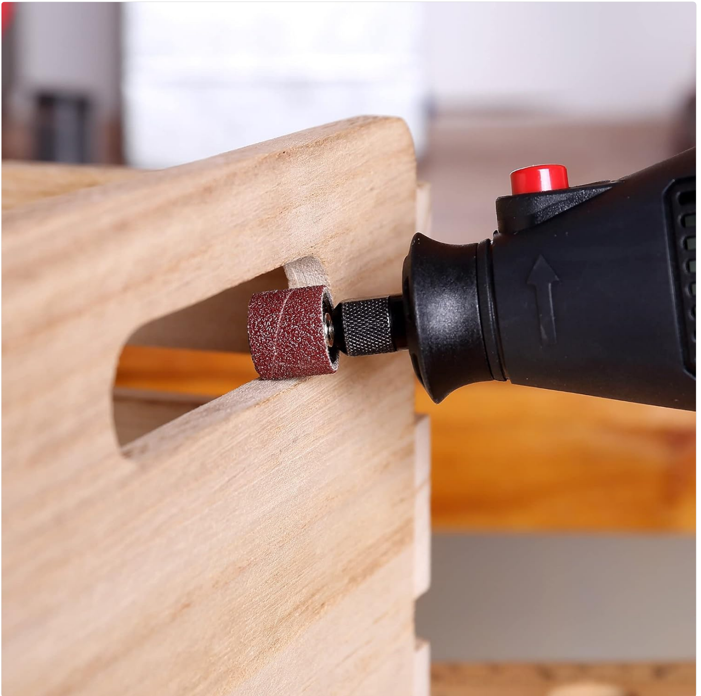
Figure 3.2: A sanding band attachment being used with a rotary tool to smooth the inside edge of a wooden crate handle, illustrating its utility for detailed sanding.
