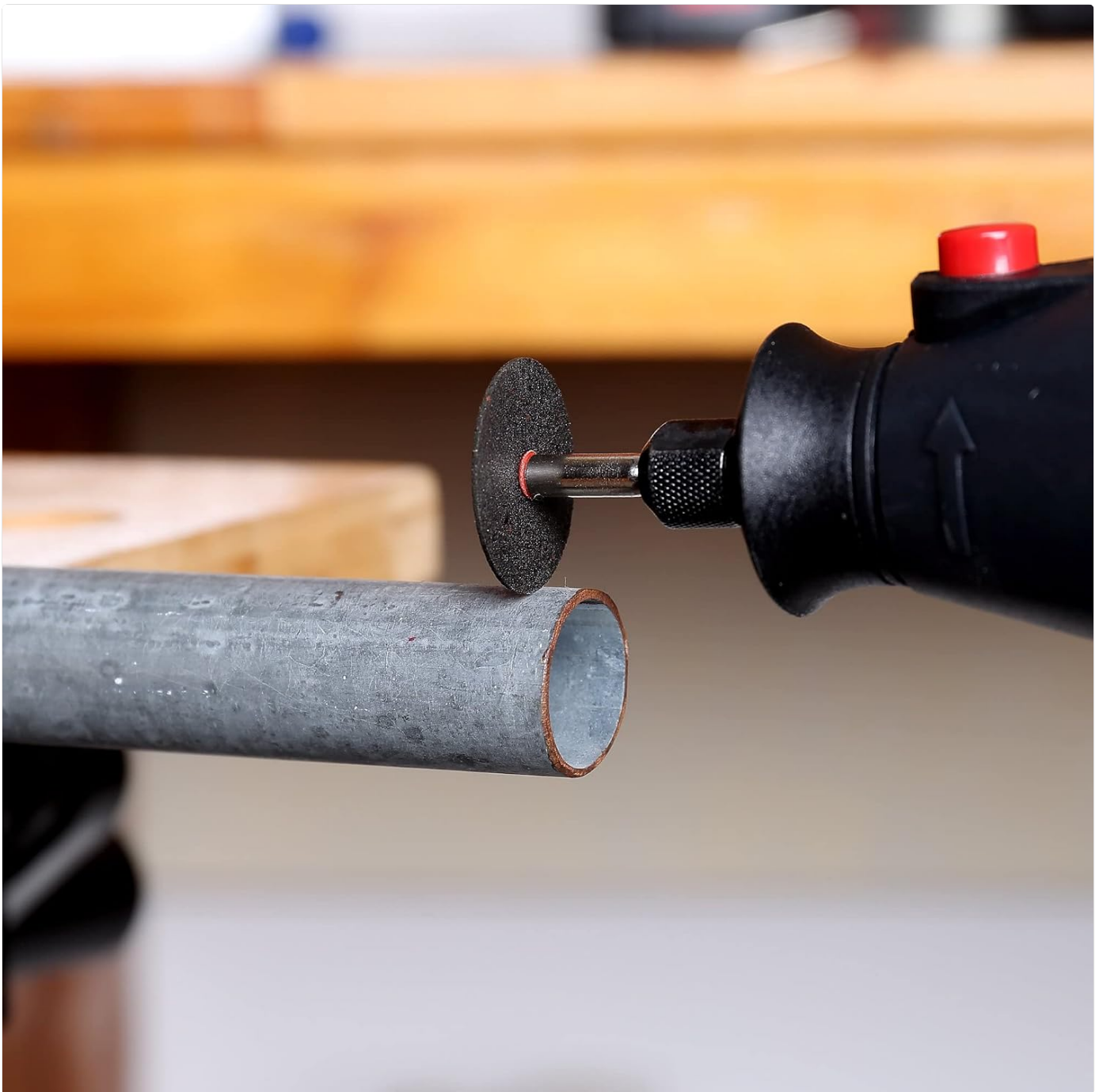
Figure 3.5: A cutting wheel attachment being used with a rotary tool to cut a metal pipe, illustrating its precision for material separation.
