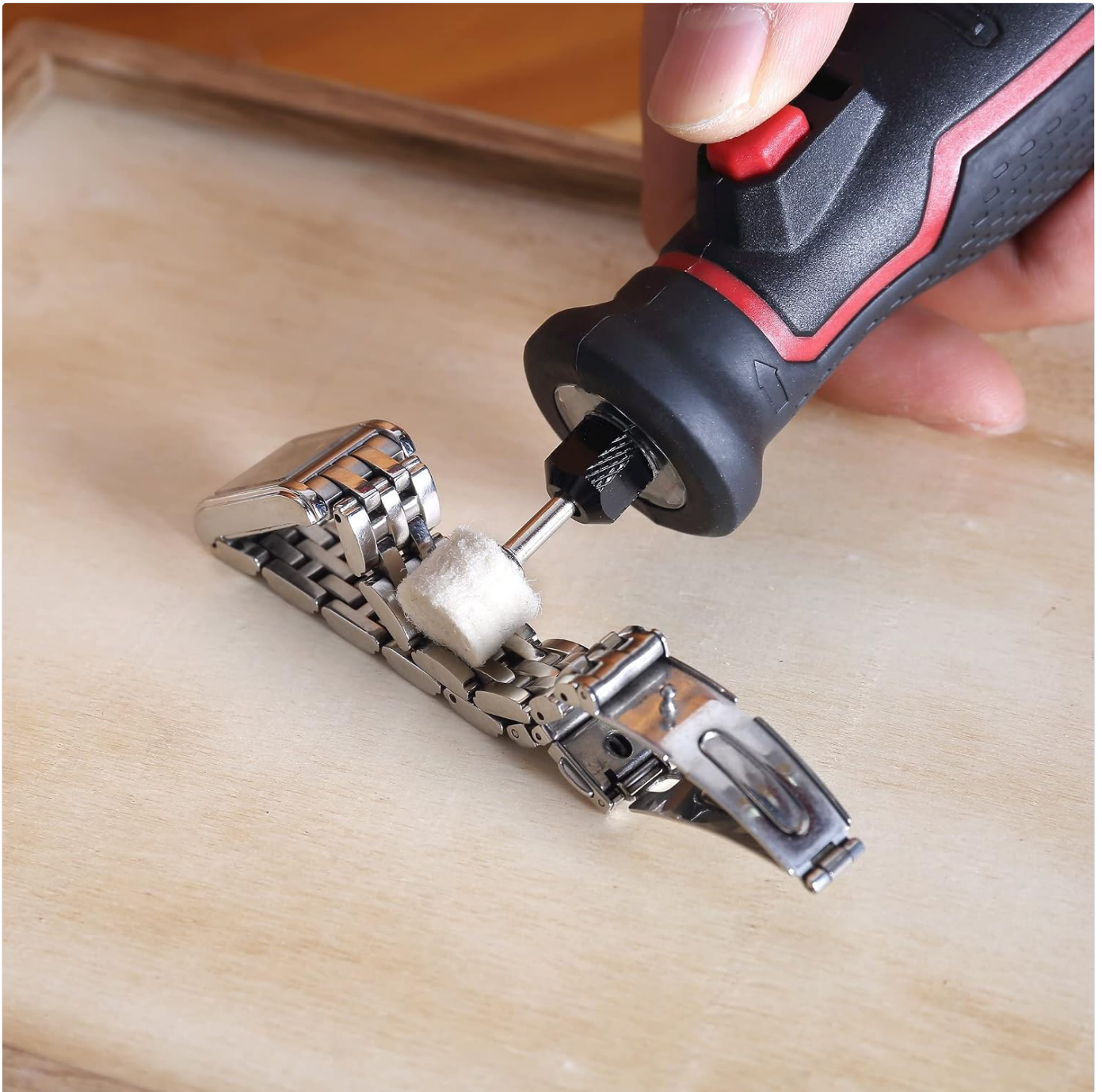
Figure 3.3: A polishing wheel attachment being used with a rotary tool to buff a metal watch band, showcasing its ability to restore shine to intricate metalwork.
