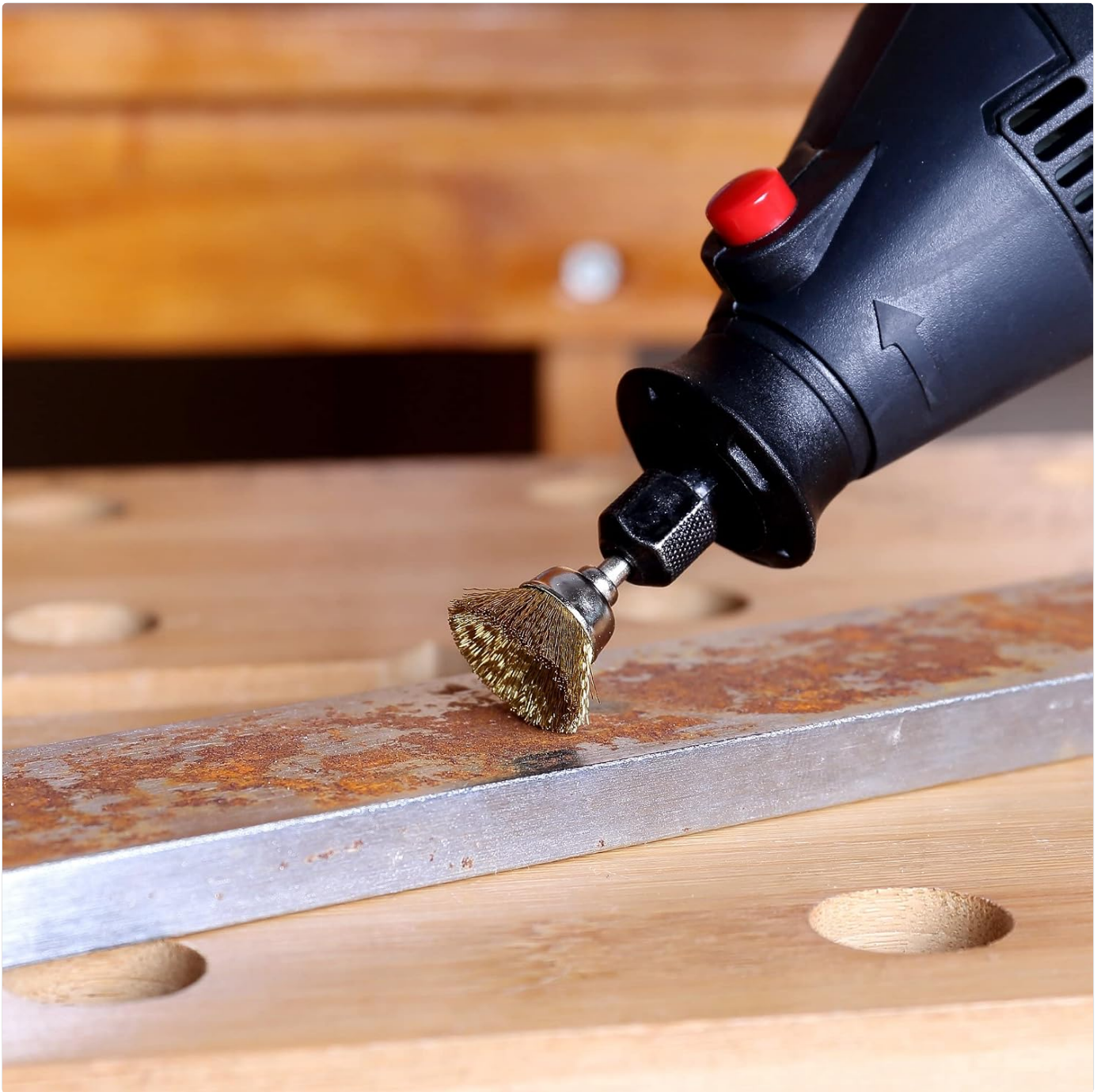
Figure 3.4: A wire brush attachment being used with a rotary tool to clean rust from a metal bar, demonstrating its effectiveness in surface preparation.
