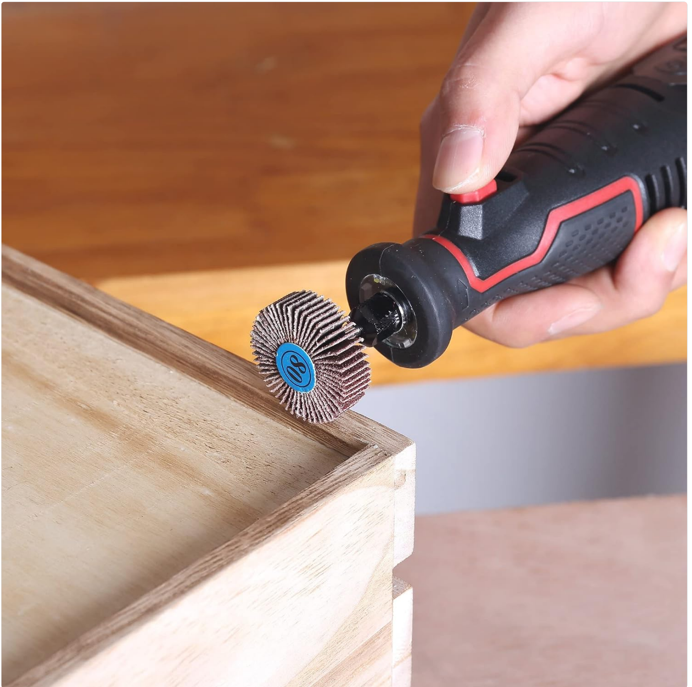
Figure 3.1: A flap wheel attachment being used with a rotary tool to smooth the edge of a wooden box, demonstrating its effectiveness on contoured surfaces.
