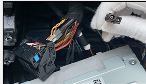
Figure 5.3: Diagram for connecting the fiber optic cable.
