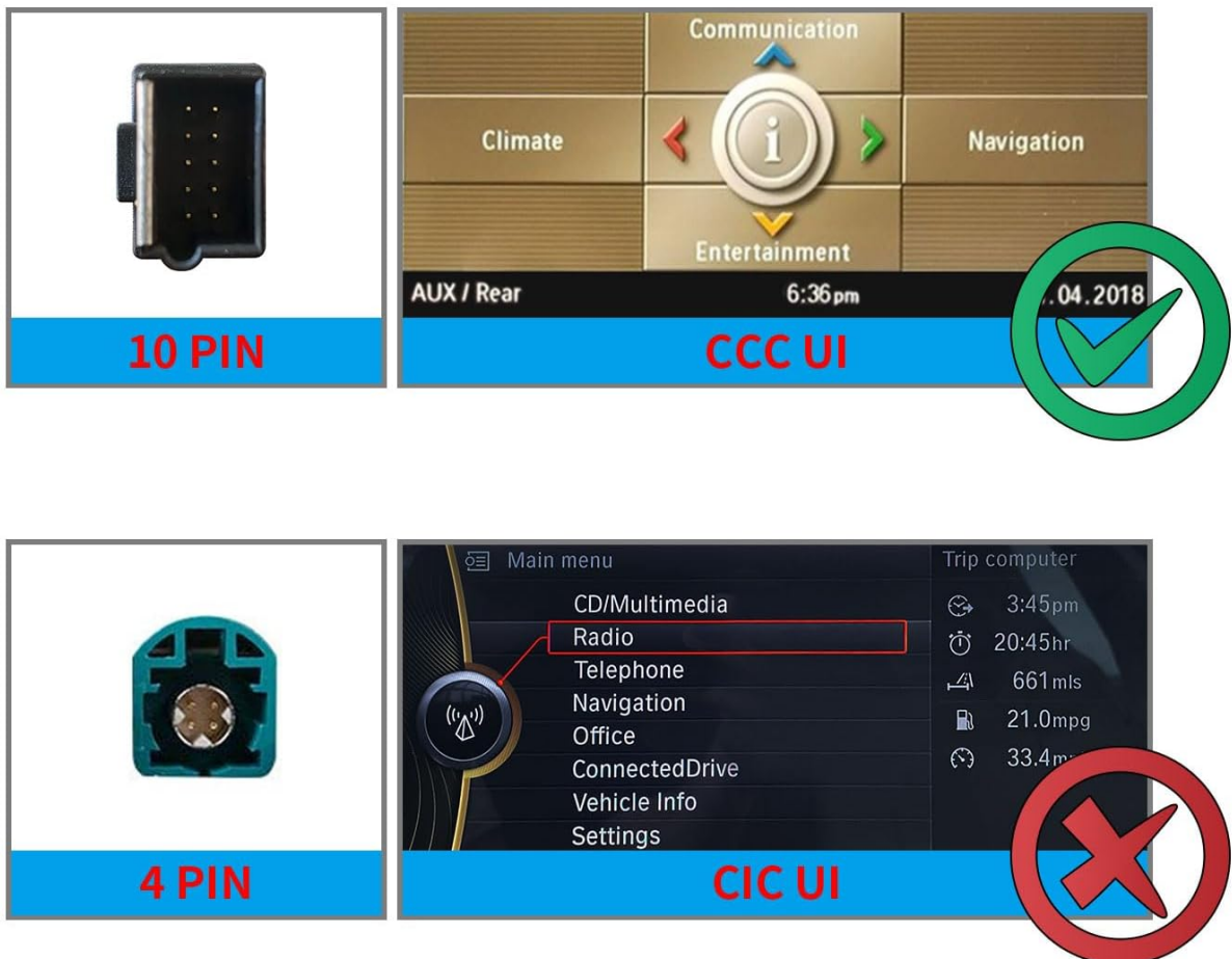
Figure 3.1: Applicable Models - Confirm your vehicle has the 10 PIN CCC UI, not the 4 PIN CIC UI.
