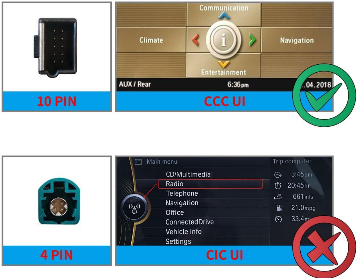
Image 4.1: Identify your car's system: The unit is compatible with CCC UI (10 PIN connector) and not with CIC UI (4 PIN connector).
