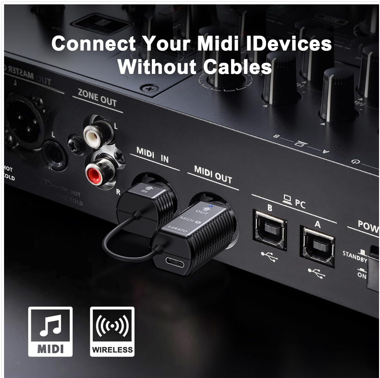
Image: The MIDI A unit connected to the MIDI IN and MIDI OUT ports of a musical instrument.
