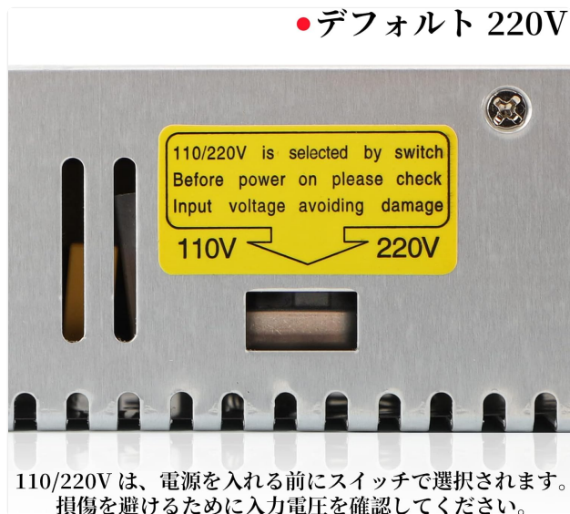
Figure 3.2.4: Important switch for selecting input voltage between 110V and 220V.
