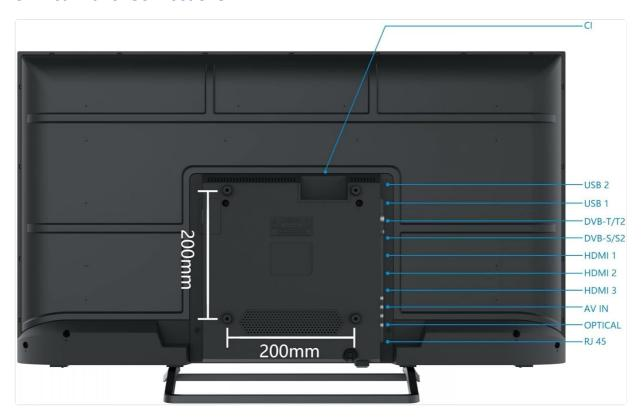
This image illustrates the rear panel of the Smart Tech 40-inch TV, highlighting its connectivity options. Labeled ports include USB 1, USB 2, DVB-T/T2, DVB-S/S2, HDMI 1, HDMI 2, HDMI 3, AV IN, OPTICAL, and RJ 45 (Ethernet). A CI (Common Interface) slot is also visible. The VESA mounting points are indicated with a 200mm x 200mm spacing.
