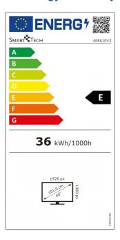
This image shows the EU Energy Label for the Smart Tech 40FA10V3 television. It indicates an energy efficiency class of E and an energy consumption of 36 kWh per 1000 hours. The label also displays the screen size as 40 inches (101 cm) with a resolution of 1920x1080 pixels. For more details, visit the official EPREL database: https://eprel.ec.europa.eu/qr/964843
