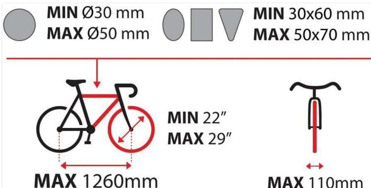
Image: Diagram detailing the minimum and maximum dimensions for compatible bicycle frames and wheels.
