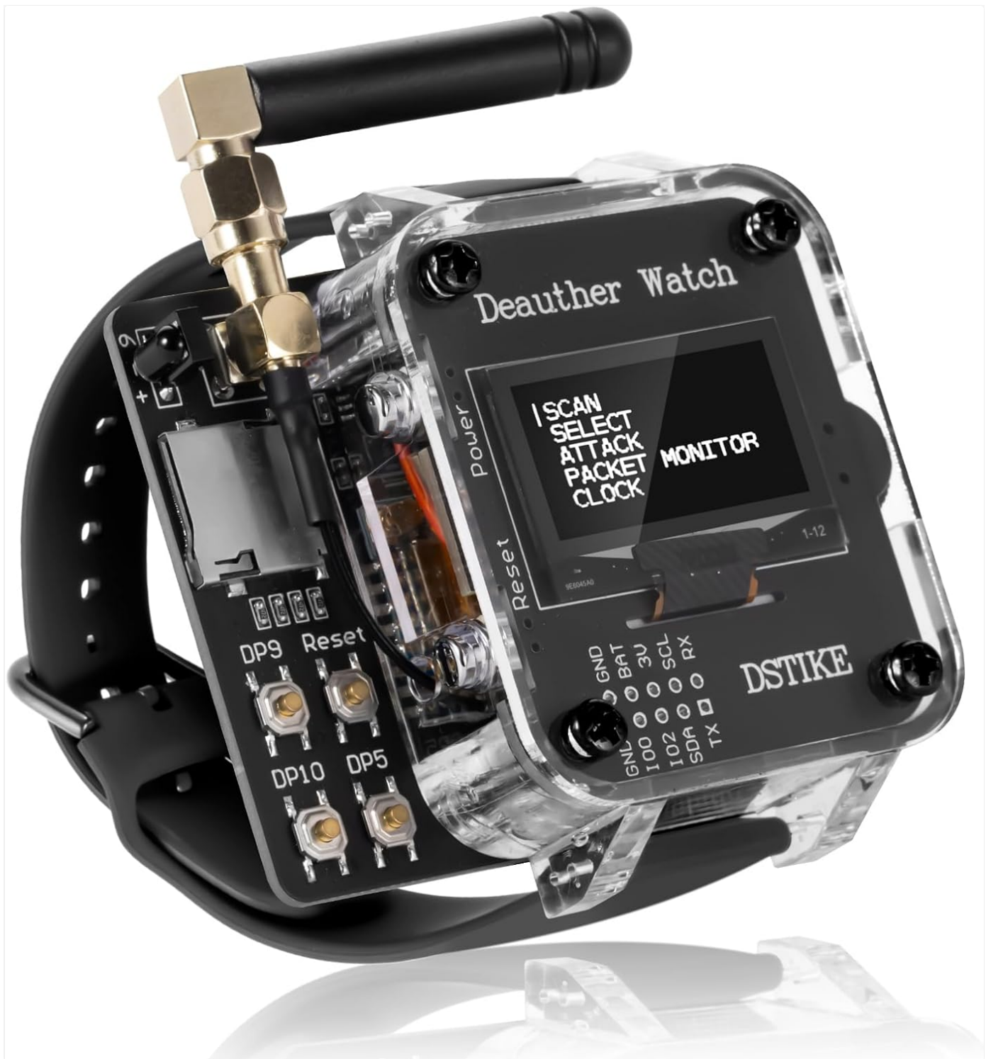
Figure 1.1: Front view of the AURSINC DSTIKE WiFi Deauther & Bad USB Watch V4, showing the display and external antenna.
