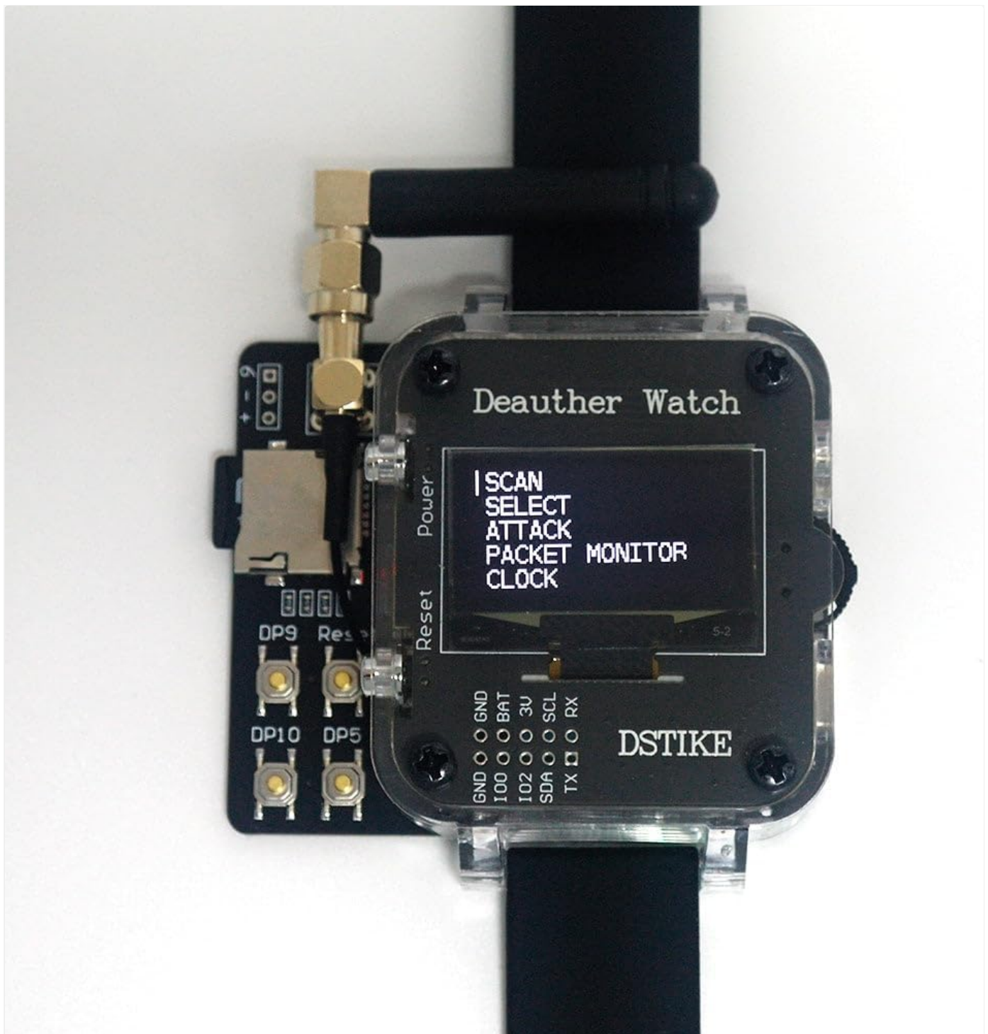
Figure 4.1: Close-up of the watch display showing menu options and the physical buttons (DP9, DP10, DP5).
