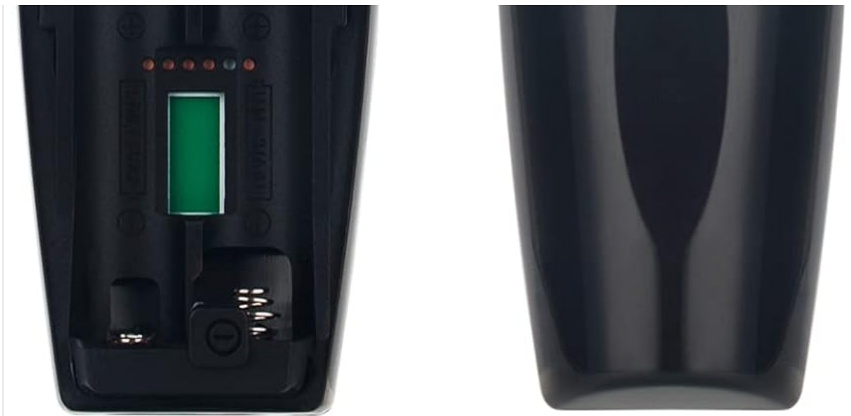
Image: Back view of the remote control, showing the open battery compartment and the 'PUSH' tab for removal.
