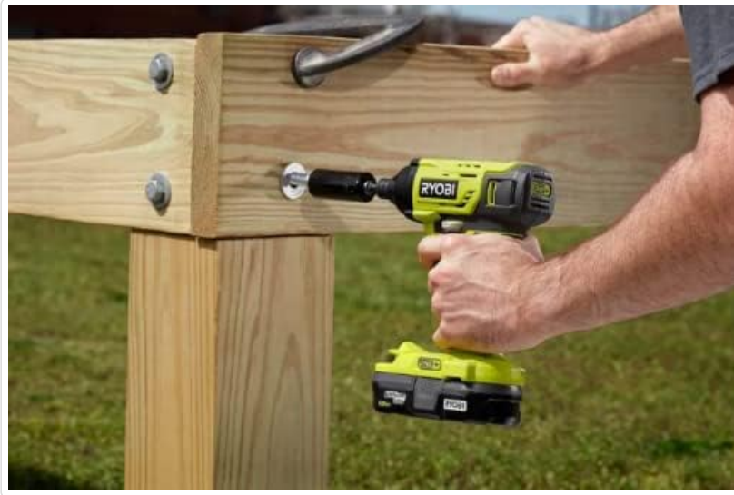
Figure 4: User operating the RYOBI Impact Driver to tighten a bolt on a wooden structure. This demonstrates the tool's application in heavy-duty fastening tasks.
