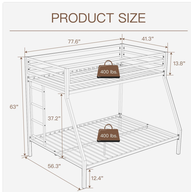
Image: Detailed diagram illustrating the overall product dimensions and the weight capacity for each bunk.
