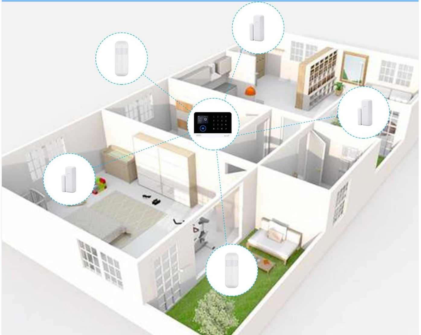
Figure 4.1: Example of sensor placement. This diagram illustrates a house floor plan with the main alarm panel centrally located and various wireless sensors (PIR and door/window) strategically placed in different rooms for optimal coverage.
