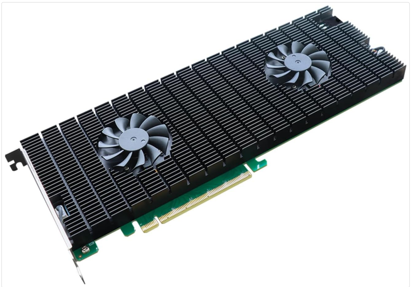
Figure 5.1: Close-up view of the HighPoint SSD7140A's multi-stage cooling solution, featuring a large heatsink and dual fans for efficient heat dissipation.
