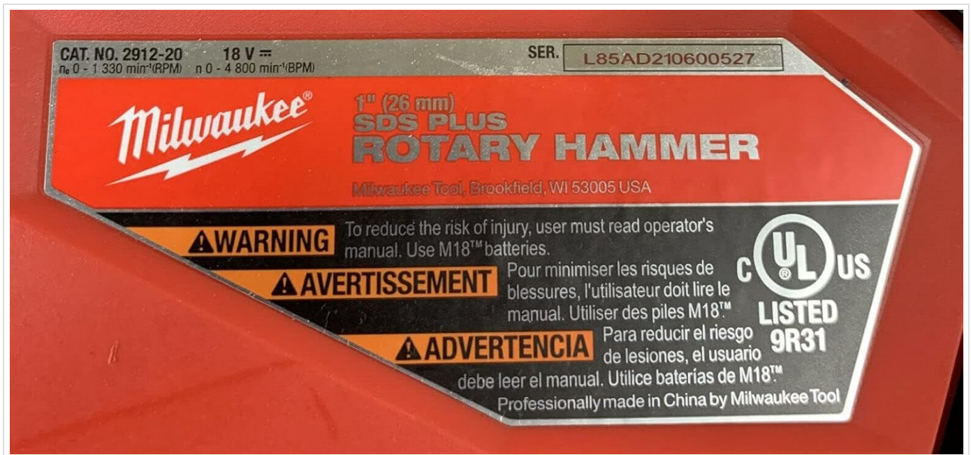
Figure 2: Product label for the Milwaukee 2912-20 Rotary Hammer. This label provides important model, serial, and safety information, including voltage and RPM specifications.
