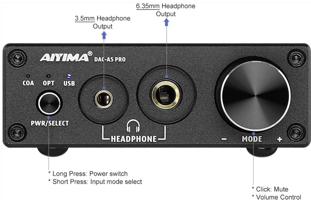
Image: Detailed view of the DAC-A5pro front panel, highlighting the power/select button, input indicators (COA, OPT, USB), 3.5mm and 6.35mm headphone outputs, and the volume/mode knob.
