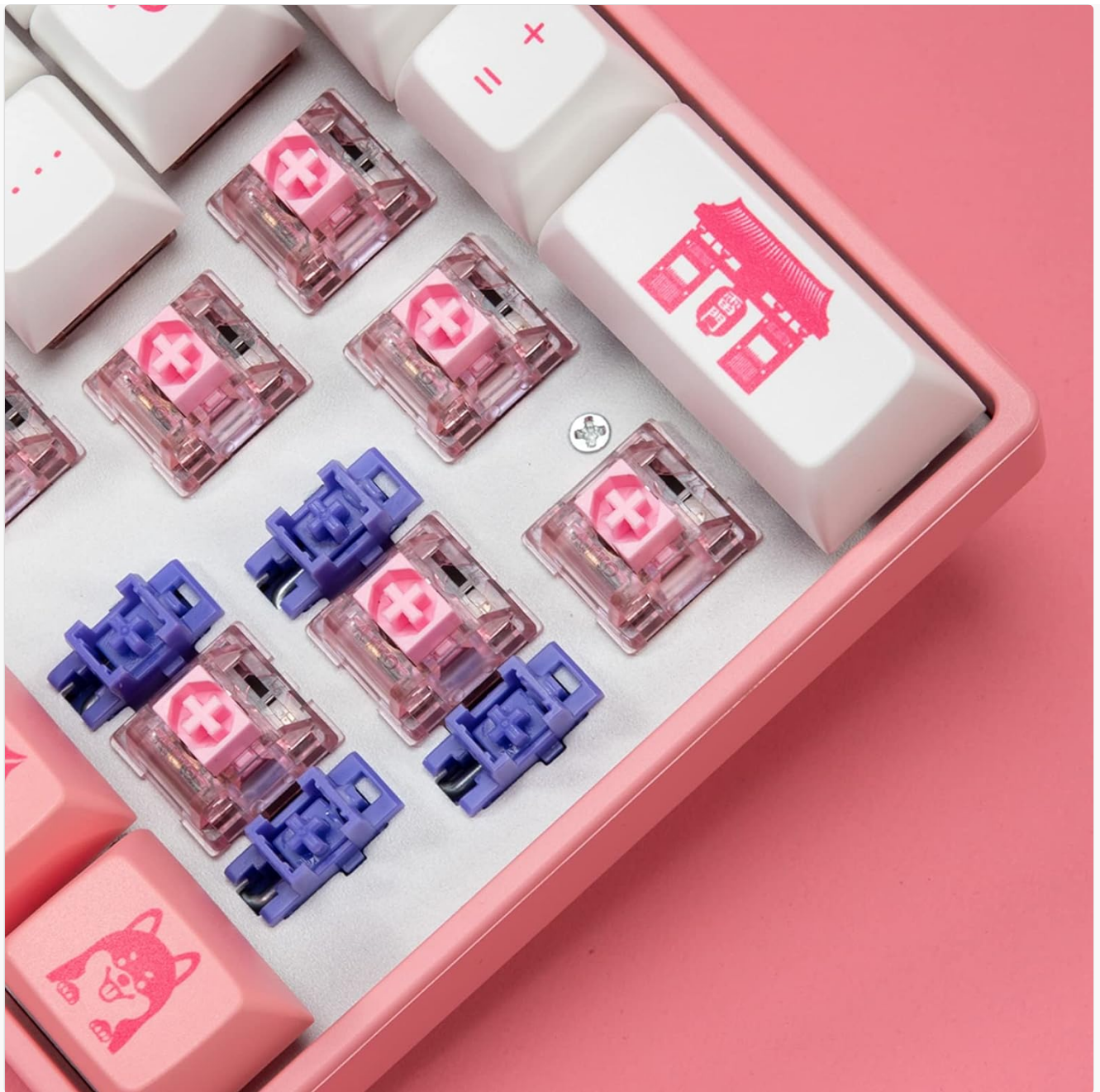
Image: Keycaps removed from the Akko 3061S, showing the hot-swappable Jelly Pink switches and stabilizers.
