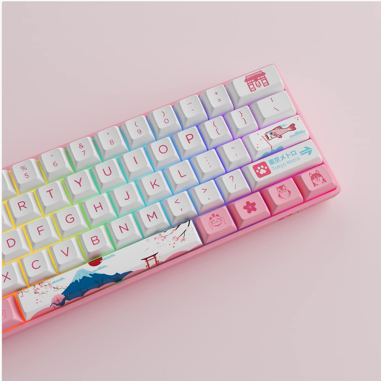
Image: Close-up of the Akko 3061S keycaps, showcasing the PBT material and dye-sublimated designs.
