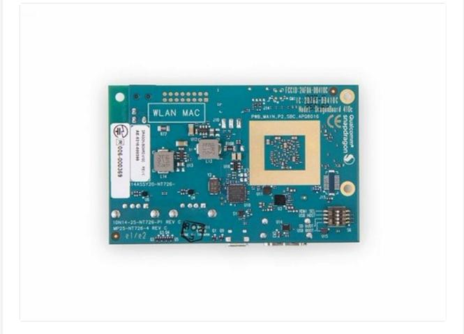
Image: Bottom view of the DragonBoard 410C, displaying regulatory markings, serial numbers, and additional surface-mounted components.
