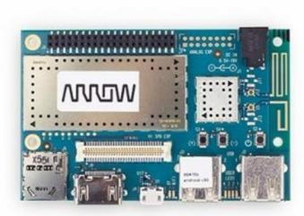
Image: Top-down view of the DragonBoard 410C, highlighting the main processor, memory, and various connectors such as USB ports, HDMI, and GPIO pins.
