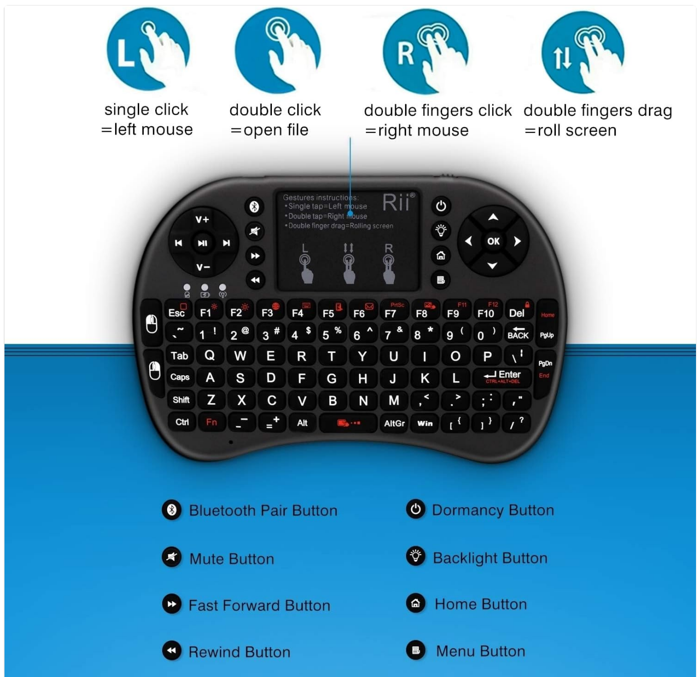
Image 5.1: Visual guide to touchpad gestures including single tap for left click, double click to open, two fingers click for right click, and two fingers drag for scrolling.
