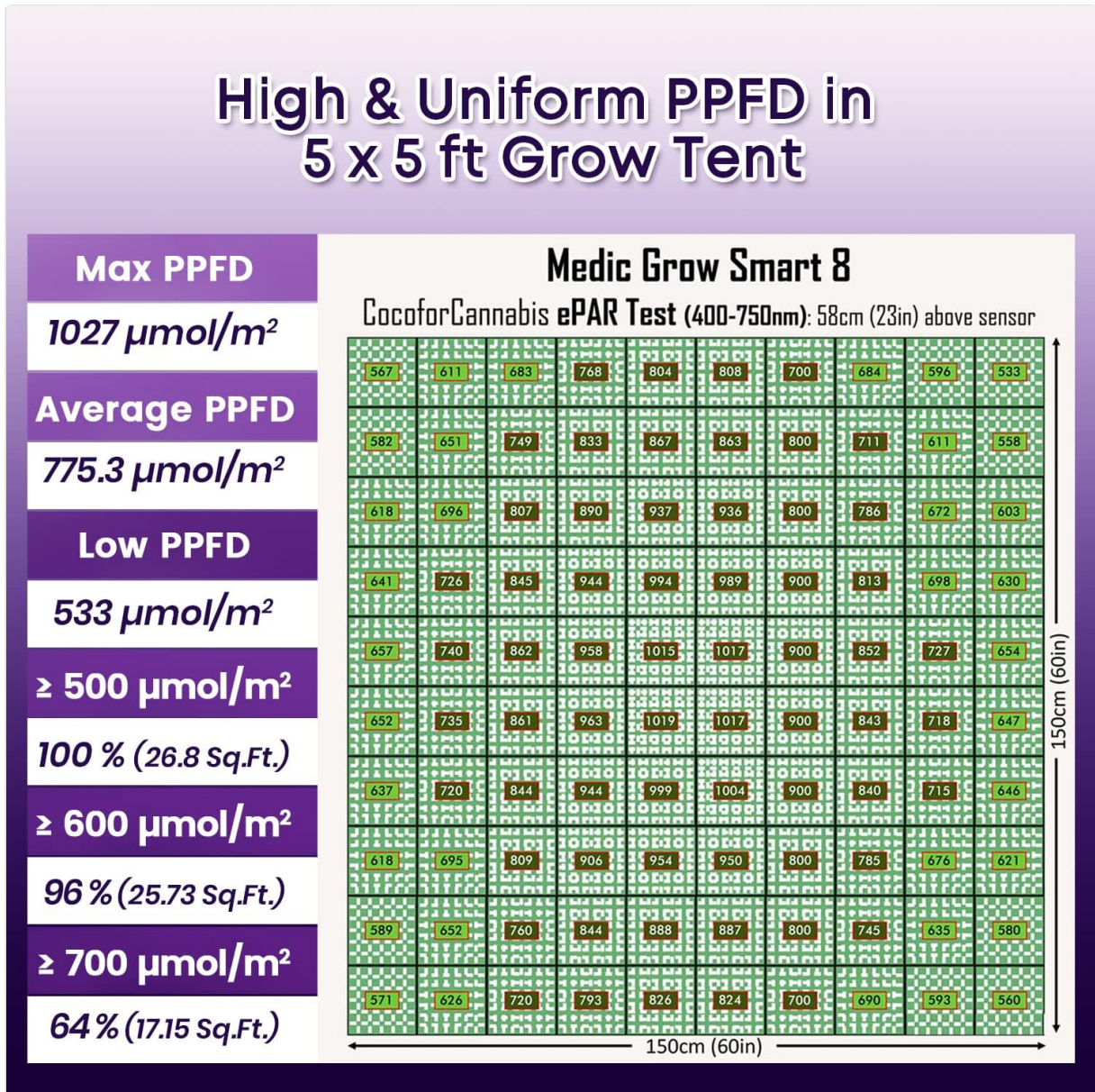
Image: PPFd map illustrating high and uniform light distribution within a 5x5 ft grow tent, showing Max, Average, and Low PPFd values.
