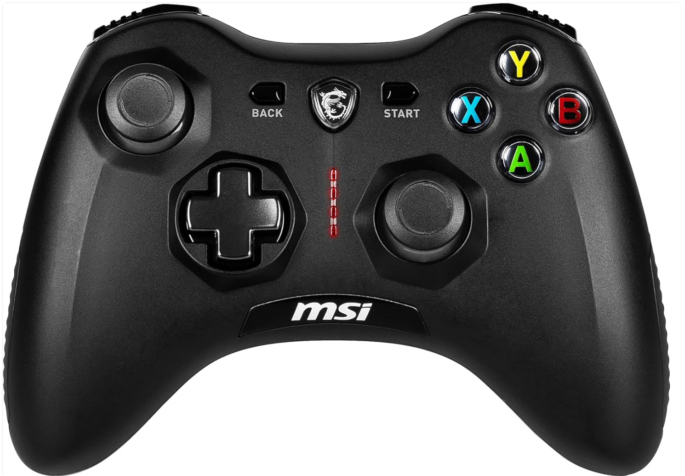
Figure 3.1: Front view of the MSI Force GC30V2 controller, showing analog sticks, D-pad, action buttons (A, B, X, Y), Back, Start, and MSI logo button.
