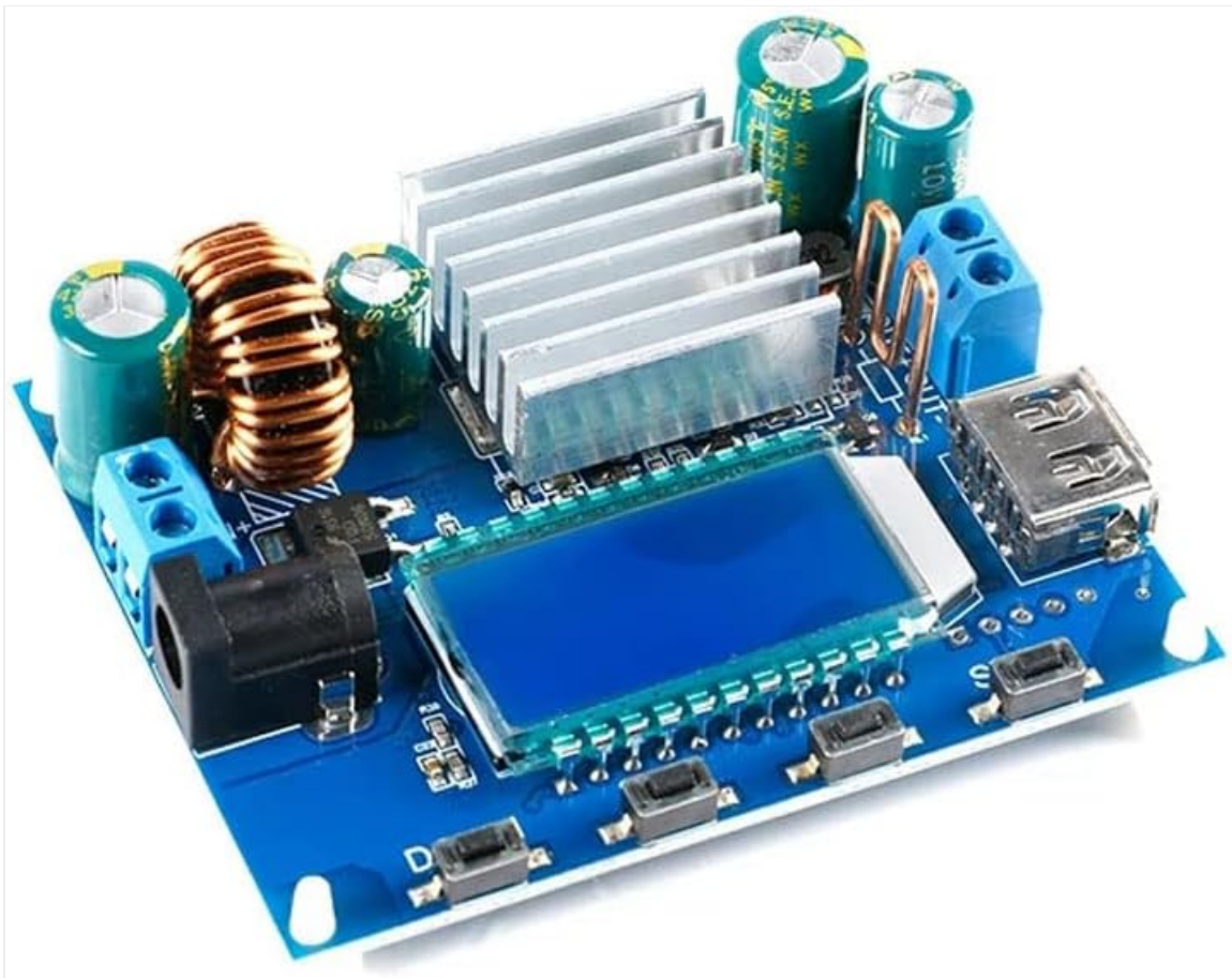
Figure 2.1: Top-down view of the XY-SK35L CNC Buck-Boost Voltage Converter module, showing the LCD screen, heat sink, inductors, capacitors, and terminal blocks.
