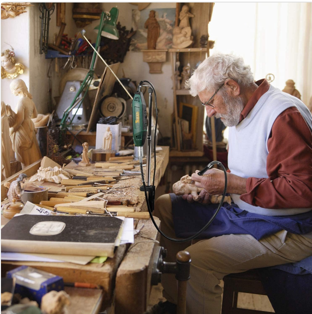
Image: An artisan using the corded rotary tool with the flexible shaft attachment for detailed wood carving, showcasing the tool's versatility for fine work.
