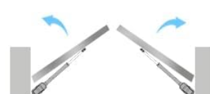
Gate Swing Out Push-to-open Installation Mode
