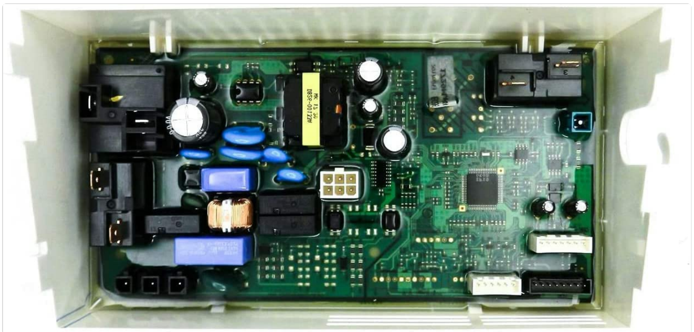
Image 1: The WEIJIA DC92-01729M Main Control Board. This image displays the overall layout and various connectors of the replacement part.
