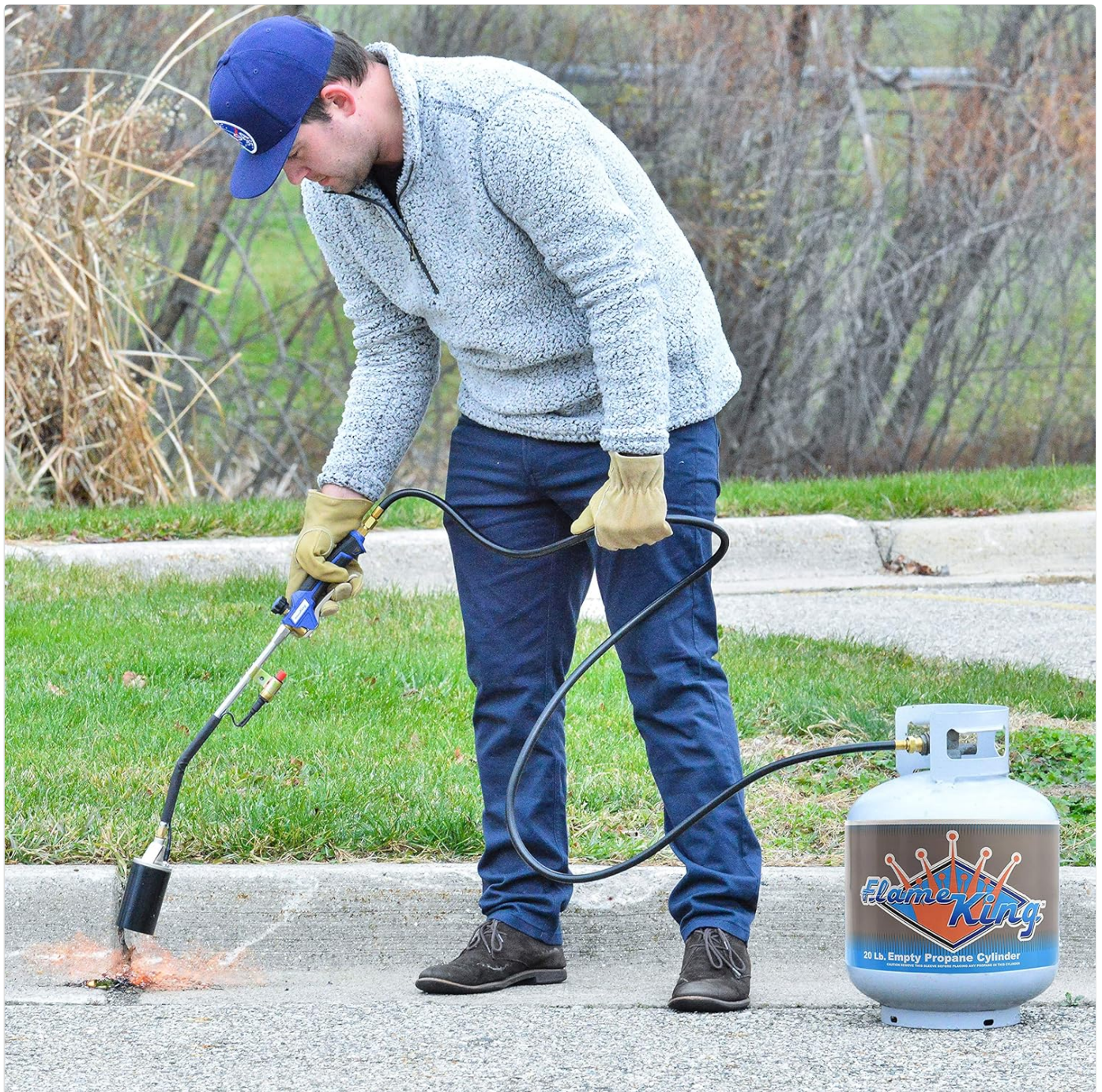
Figure 1: POL fittings are reverse thread. Tighten by turning left ('Lefty Tightly, Righty Loosey').
