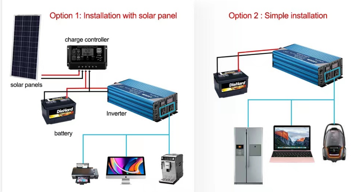
Image 4.2: Two connection options: Option 1 shows installation with a solar panel, charge controller, battery, and inverter. Option 2 illustrates a simple installation directly connecting the inverter to a battery to power household appliances.
