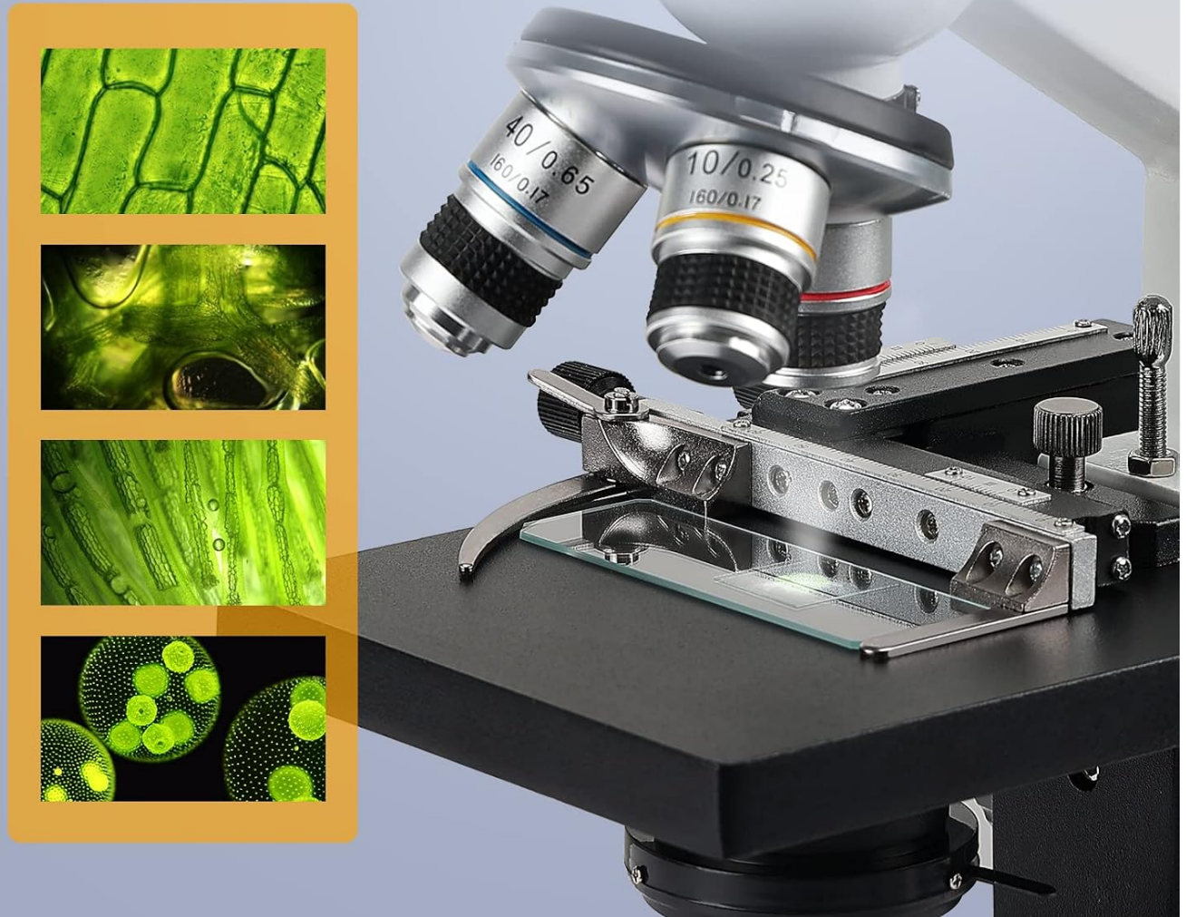
Image 4.2: Detail of the objective lenses mounted on the revolving nosepiece, positioned above the mechanical stage.
