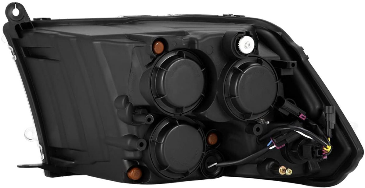
Image: Rear view of a removed factory headlight assembly, showing wiring harnesses and bulb sockets.
