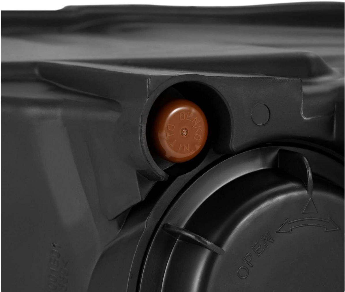
Image: Close-up of the rear of the new headlight assembly, showing the signal light socket being installed.
