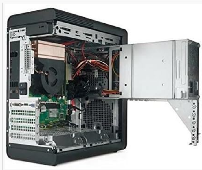
Image 3.1: Internal view of the Dell XPS 8930 Tower Desktop with the side panel removed, showing the motherboard, CPU cooler, and graphics card.
