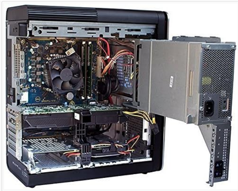
Image 3.2: Internal view of the Dell XPS 8930 Tower Desktop with the power supply unit swung out, providing better access to the internal components for maintenance or upgrades.
