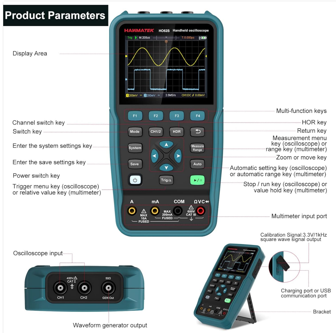
Figure 5.1: Front panel and side view with labeled components.
